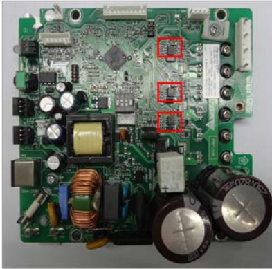
IGBT Drivers Location
